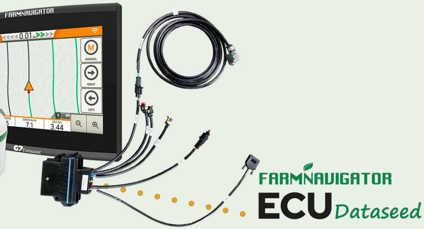
ECU controlling the automated weeder directly on the hydraulic electrovalves
